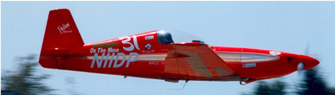
The Polen Special first appeared at the Experimental Aircraft Association's (EAA) Oshkosh air show more than 35 years ago, stunning everyone with its beauty, speed, efficiency and innovation. Powered by a small 180 horsepower engine, the Polen Special is capable of top speeds exceeding 320 mph at altitudes over 21,000 feet. The Special's extraordinary efficiency allows jet-like cruise speed using only 8.5 gallons of fuel per hour.
